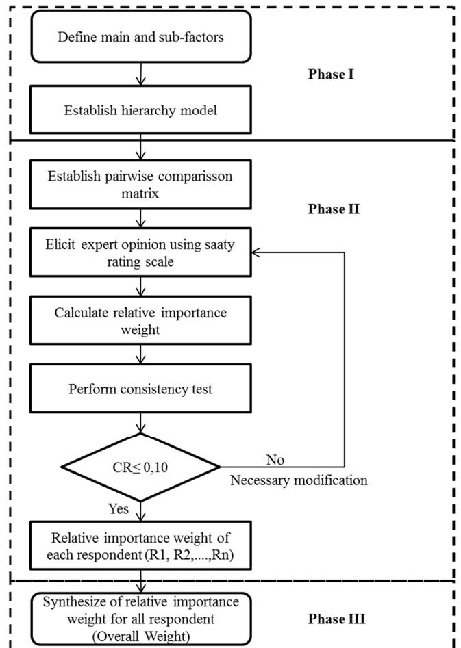
Fig. 1 Flowchart of the AHP method
