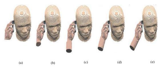
Fig. 4. The hand phantoms with different wrists: (a) no wrist, (b) 3cm long wrist, (c) 10cm long wrist (d) 10cm long 15 degrees tilted wrist, and (e) 10cm long 30 degrees tilted wrist
