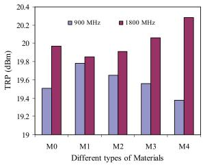
Fig. 3. Effect of hand material properties on radiation performance at 900 MHz and 1800 MHz
