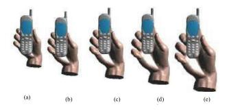
Fig. 6. The hand phantom different hand sizes for evaluating the influence of different mobile phone antenna performance: (a) 80 %, (b) 90 %, (c) 100 %, (d) 110 %, and (e) 120 % of the average hand size
