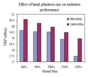
Fig. 7. Effect of hand phantom sizes on radiation performance at 900 MHz and 1800 MHz
