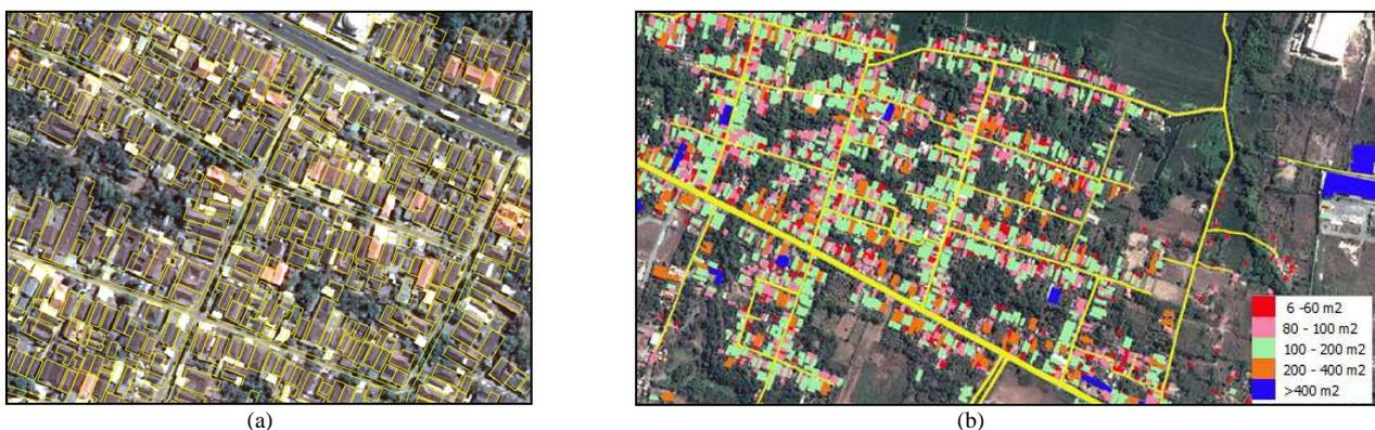
Fig. 6 Assessing feature extracted from Pleiades imagery for large scale map using the reference map shows building and road delineation
