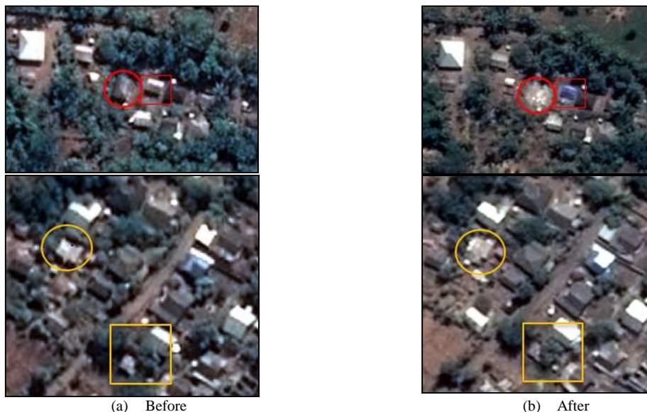
Fig. 10 Building loss detected after Lombok earthquake from Pleiades imagery acquired on a) 1 May 2018 and b) 7 August 2018
