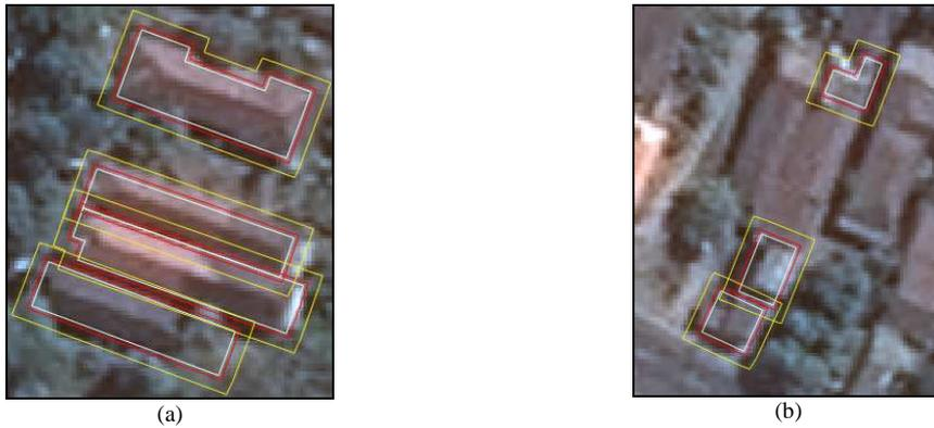
Fig. 7 Delineation accuracy for building from the reference map in white and red as tolerance accuracy for 0.5m from reference (for level 2 map scale standard), yellow as tolerance accuracy for 2m from the reference map (for level 3 map scale standard), while image b) shows the building delineation for area less than 45 m<sup>2</sup>
