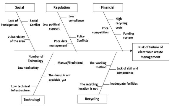
Fig. 3 Fishbone risk diagram failure e-waste management process
