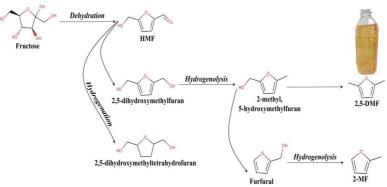
Fig 1. Converting diagram of carbohydrates into DMF
