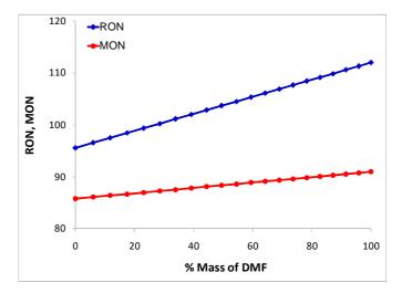
Fig 3. RON and MON of DMF-gasoline RON95 blends as a function of mass percentage of DMF  $\,$
