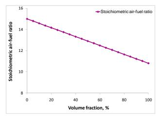
Fig 4. Stoichiometric air-DMF-gasoline RON95 ratio as a function of DMF volume fraction
