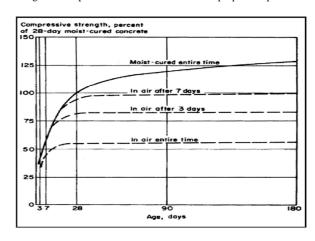
Fig.14 Effects of curing conditions on fc'[21]
