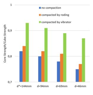
Fig. 8 Effects of compaction [11]
