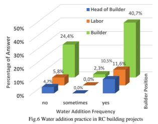
Fig. 6 presents the finding of water addition practice quantitatively. Water addition is a practice that is conducted by the builders who find their concrete mix has been dry after a couple of time counted since the concrete setting time is finish. Some builders explain that when they add water, they also add cement. However, this practice will result in increasing of un-homogeneity of concrete mix and decreasing of concrete strength.
