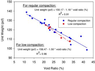
Fig. 9 Effect of improper compaction on concrete weight [19]
