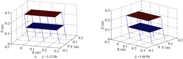
Fig. 4 Two lowest modes of the structure
