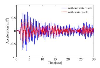
Fig. 10 Acceleration response at point A' under El-Centro earthquake
