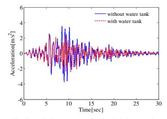
Fig. 13 Acceleration response at point B' under Kobe earthquake
