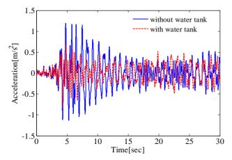
Fig. 11 Acceleration response at point B' under Hachinohe earthquake
