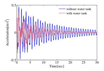
Fig. 7 Acceleration response at point B' under impulsive excitation
