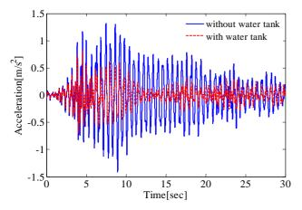
Fig. 12 Acceleration response at point A' under Hachinohe earthquake
