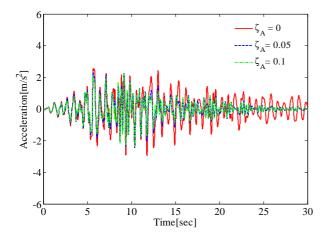
Fig. 15 Acceleration response at point B' with a variation of  $\zeta$
