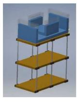
Fig. 1 A two-storey building model with u-shape water tank
