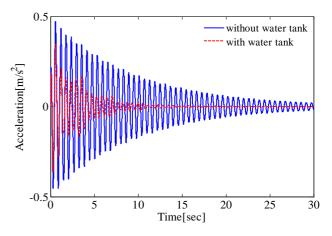
Fig. 8 Acceleration response at point A' under impulsive excitation
