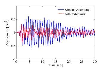
Fig. 9 Acceleration response at point B' under El-Centro earthquake
