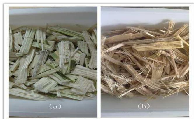
Fig. 6 Photograph of dried oil palm frond using: (a) Spouted bed (b) Direct sunlight
