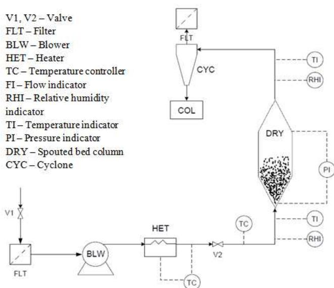
Fig. 1 Schematic diagram of spouted bed dryer
