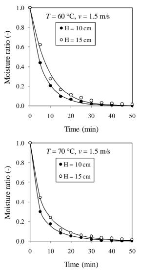
Fig. 5 Effect of initial bed height on drying kinetics of oil palm fronds
