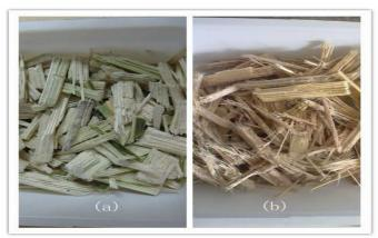
Fig. 6 Photograph of dried oil palm frond using: (a) Spouted bed (b) Direct sunlight
