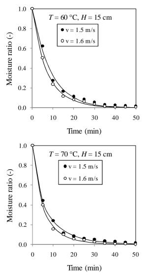
Fig. 4 Effect of inlet air velocity on drying kinetics of oil palm fronds
