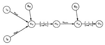
Fig. 3 Gravity Artificial Neural Network (GANN) used by Black [6]
