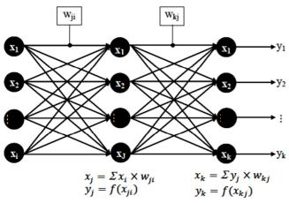
Fig. 2 Multilayer Feedforward Neural Network (MLFFNN)
