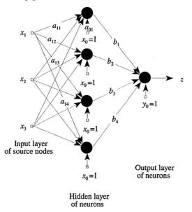
Fig. 4 Neural Network Architecture used by Mozolin et al. [15]
