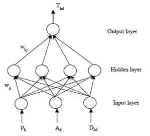
Fig. 5 Neural Network Architecture used by Yaldi et al. [11]
