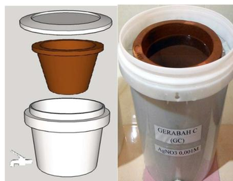
Fig 2. Ceramic Water Filter Pot Models
