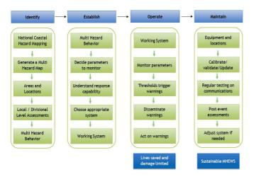
Fig. 2 Schematic representation of MHEWS
