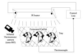
Fig. 4 Infrared heater drying of Pla-duk-ra
