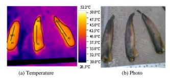
Fig. 6 Temperature reading and distribution of heat in Pla-duk-ra dried under open sun
