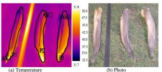
Fig. 12 Temperature reading and distribution of heat in Pla-duk-ra dried using hot-air tray drying
