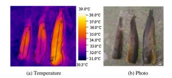
Fig. 8 Temperature reading and distribution of heat in Pla-duk-ra dried under shade drying
