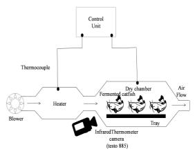
Fig. 5 Hot-air tray drying of Pla-duk-ra
