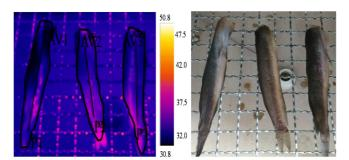
(a) Temperature (b) Photo Fig. 10 Temperature reading and distribution of heat in Pla-duk-ra dried using infrared heater drying
