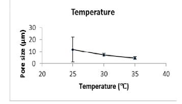
Fig. 8 Effect of temperature on microcarrier pore size
