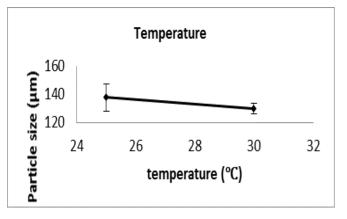
Fig. 7 Effect of temperature on microcarrier particle size
