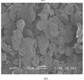
Fig. 4 SEM morphology of the PCL micro-carriers. The concentration of camphene was varied: Camphene ratio (a) 0%, (b) 10%, (c) 20%, (d) 40% and (e) 60%.
