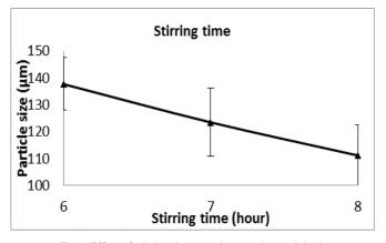
Fig. 9 Effect of stirring time on micro-carrier particle size
