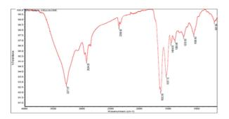
Fig. 6 FTIR spectra for bacterial cellulose (BC CM<sup>-1</sup>)
