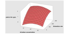
Fig. 4 The 3-Dimensional surface plot showing the interaction between carbon sources concentration and aeration rate leading to yield of BC.
