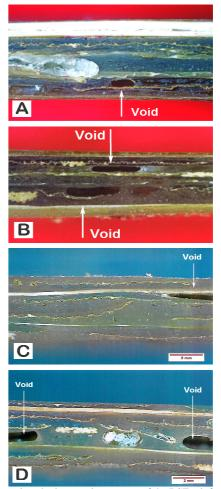
Fig. 3 Cross-sectioned microscopic structure of the RSF-reinforced polymer composite at 10% (A), 20% (B), 30% (C) and 40% (D) fibre loading ( $RSF_{NaOH}$ ).
