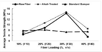
Fig. 1 Ultimate tensile strength exhibited by the RSF-reinforced composites at various fibre loadings.
