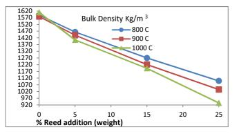
Fig. 7 Effects of % Reed addition on bulk dry density of fired clay bricks exposed to different burning temperature
