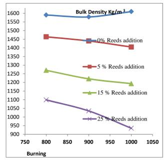
Fig. 8 Effects of burning temperature on bulk dry density of fired clay bricks containing different % Reed addition
