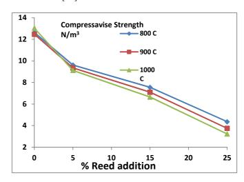
Fig. 11 Effects of % Reed addition on compressive strength of fired clay bricks exposed to different burning temperature
