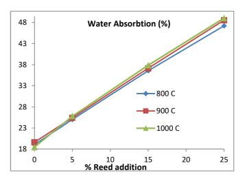
Fig. 9 Effects of % Reed addition on water absorption of fired clay bricks exposed to different burning temperature
