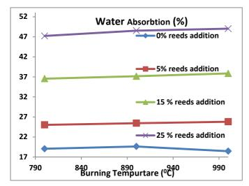
Fig. 10 Effects of burning temperature on water absorption of fired clay bricks containing different % Reed addition
