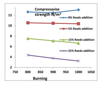
Fig. 12 Effects of burning temperature on compressive strength of fired clay bricks containing different % Reed addition.
