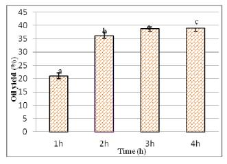
Fig. 3 Effect of incubation time on aqueous enzymatic oil extraction from cashew nut.
