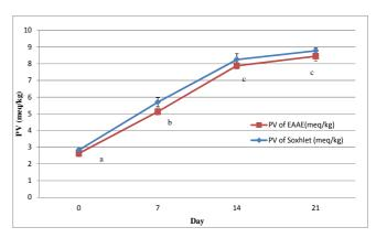
Fig.4 Peroxide value of cashew nut oil extracted by Soxhlet and EAAE method and stored at  $60^{\circ}C$
