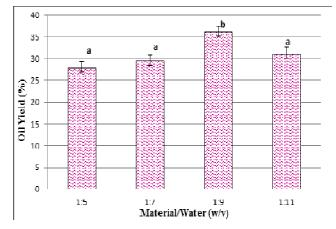
Fig.1 Effect of material/water ratio on aqueous enzymatic oil extraction from cashew nut.
