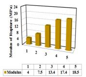
Fig. 6 Concrete mix type and increase in flexural strength with steel fiber impact.
