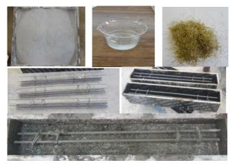
Fig. 2 Silica fume, superplasticizer, steel fiber, and steel reinforcement used.
