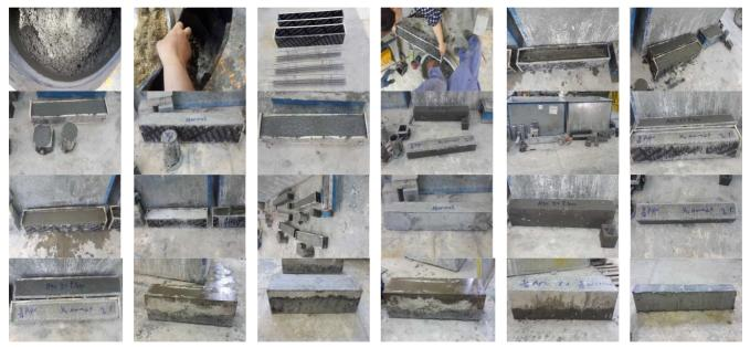
Fig. 4 Preparation, mixing, casting and curing procedure.
