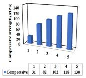
Fig. 5 Concrete mix type and increase in compressive strength with steel fiber impact.
