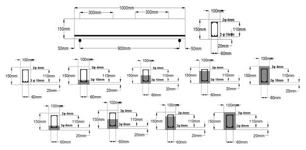
Fig. 3 Details of beam specimens, overall dimensions, reinforcement details, loading positions.
