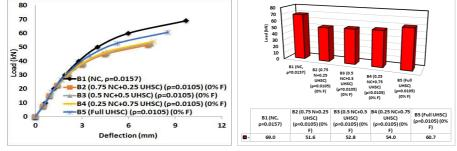
Fig. 14 Load-deflection curve for hybrid concrete beam (1,2,3,4 and 5) with steel fiber (0%)
