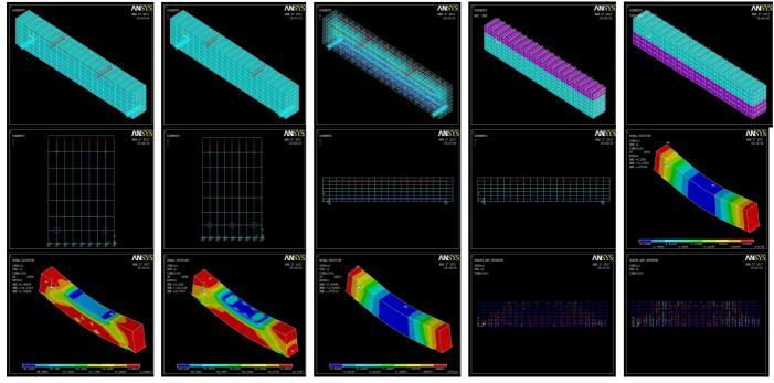
Fig. 27 Finite element meshing, boundary condition, loading arrangement, crack and stress contour.
