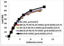
Fig. 15 Load-deflection curve for hybrid concrete beam (1,6,7,8 and 9) with steel fiber (1.0%)
