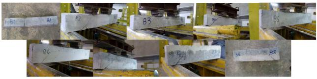
Fig. 10 Shear failure and crack propagations of the tested beams
