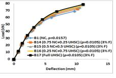
Fig. 17 Load-deflection curve for hybrid concrete beam (1,14,15,16 and 17) with steel fiber (2.0%)
