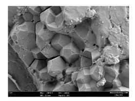
Fig. 6. Polyhedral crystalline solids between the rectangular blocks at 3000X magnification.
