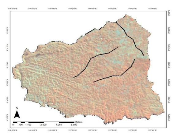
Fig. 2 Color composite result of 567 bands from Landsat 8 image and lineament interpretation (black dotted lines).
