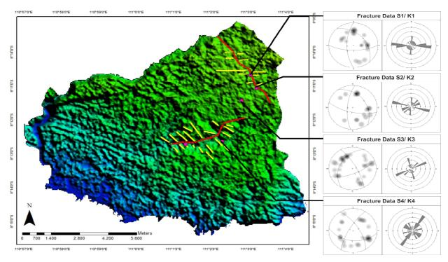
Fig. 5 Joint/fracture data analysis in stereography projection, lineament analysis (red line) and shifting ridge analysis (yellow line) based on SRTM image.
