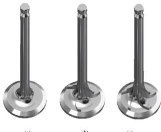
(a) (b) (c) Fig. 1 Design of Fin Adding on Intake Valve. a. original, b. 3 fins, c. 5 fins
