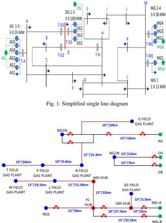
Fig. 2: Gas line configuration
