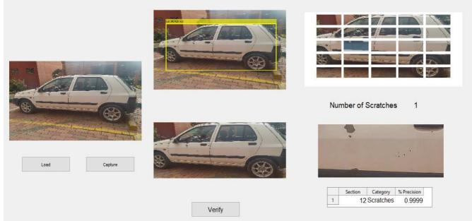
Fig. 13 Scratch identification case.
