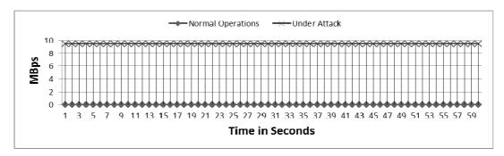
Fig. 7 Windows 10 Home Bandwidth Consumption Before and During DoS Attack on SeND
