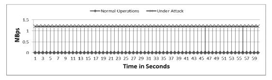
Fig. 8 Ubuntu 16.04 Bandwidth Consumption Before and During DoS Attack on SeND
