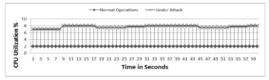
Fig. 5 Windows 10 Home Processor Consumption Before and During DoS Attack on SeND
