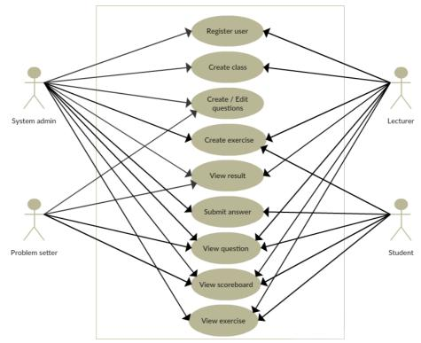
Fig. 1 The Auto-marking programming exercise system use case diagram.
