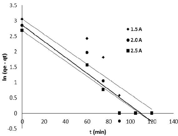
Fig. 4. First order modelling of Fe electrocoagulation
