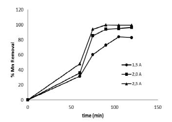
Fig. 3 . Decreased percentage of Mn content by electrocoagulation current and process time variations
