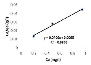
Fig. 6. Langmuir Fe - Adsorption Isotherm
