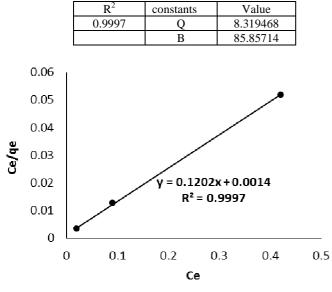
Fig. 7 Langmuir Mn - Adsorption Isotherm
