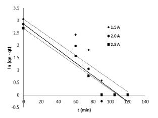
Fig. 4. First order modelling of Fe electrocoagulation
