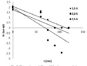
Fig.5. First order modelling of Mn electrocoagulation
