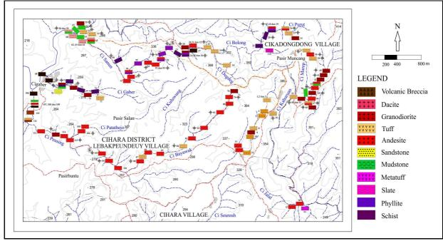
Fig. 2. Field observation of metamorphic rock distribution in Bayah Geological Complex
