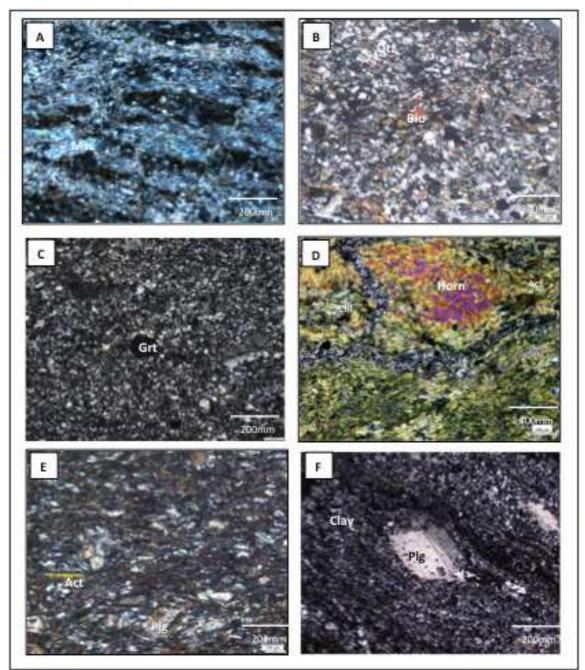
Fig. 4. These represent metamorphic rock in Bayah area showed good foliation. (A) Muscovite schist, (B) Biotite - Muscovite schist, (C) Garnet Biotite schist, (D) hornblende schist, (E) Actinolite Schist and (F) Quartz Slate.
