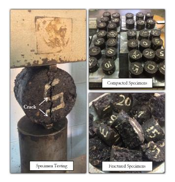
Fig. 5 Indirect tensile strength test
