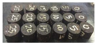
Fig. 3 Marshall specimens
