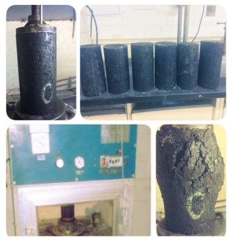
Fig. 8 Uniaxial repeated loading test
