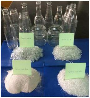
Fig. 2 Crushed waste glass
