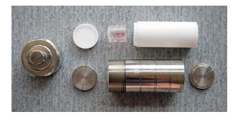
Fig. 4. Autoclave reactor (250 ml)
