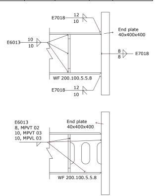
Fig. 4. Type of weld at the end of each model, a standard link and a modified link  $% \left( {{{\rm{A}}_{\rm{B}}}} \right)$
