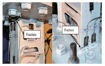
Fig. 10 Fracture on the MPVT02 model
