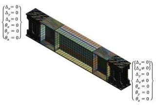
Fig. 6 Boundary conditions with restraints  $\Delta_x = 0$  and without restraints the axial force  $\Delta_x \neq 0$
