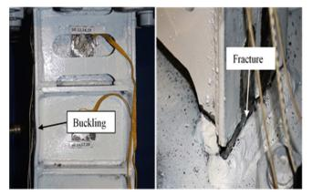
Fig. 11 Fracture and local buckling on the MPVT03 Model
