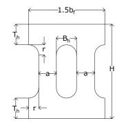
Fig. 1 Supplemental double stiffeners limitations
