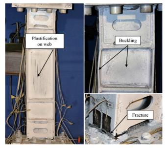
Fig. 12 Fracture and local buckling on the MPVL03 Model
