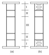
Fig. 8 Zoning observed on (a) link standard, and (b) link with supplemental double stiffeners
