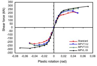
Fig. 13 A comparison of backbone curve of the models
