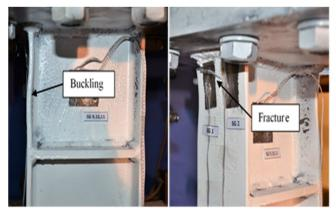
Fig. 9 Fracture and local buckling on the Standard Model
