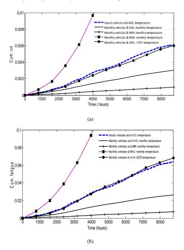
Fig. 7 Cumulative damage; (a) rutting and (b) fatigue
