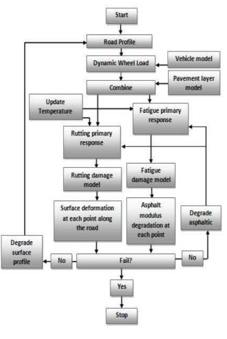
Fig. 1. Pavement Performance Model
