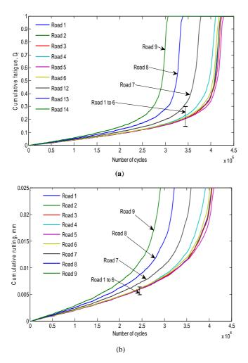
Fig. 6 Cumulative damages, (a) fatigue and (b) rutting
