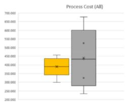
Figure 7. Box-and-Whisker plot of Overall Process Cost in PhP/m2 (left box for method A and right box for method B)
