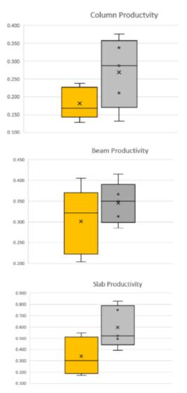
Fig. 5 Box-and-Whisker plots of Labor Productivity in m2/manhours (left box for method A and right box for method B)
