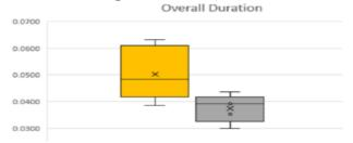
Fig 9 Box-and-Whisker plot of Total Overall Duration over Total Area in Days/m2 (left box for method A and right box for method B)
