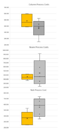
Fig. 6 Box-and-Whisker plot of Process Cost in PhP/m2 (left box for method A and right box for method B)
