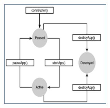
Figure 2: MIDlet life cycle-the three abstract methods startApp(), pauseApp(), and destroyApp() must be implemented.
