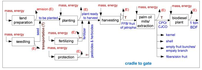
Fig.1. The system boundary of this study
