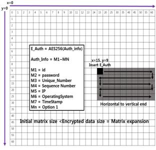
Fig. 4 E\_Auth Insertion Process
