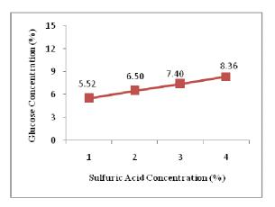
Fig. 1 Glucose concentrations after acid hydrolysis process
