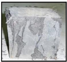
Fig. 5 Failure mode of specimen RPC with steel fibers
