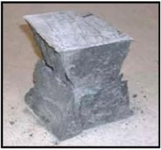
Fig. 6 Failure mode of specimen normal concrete
