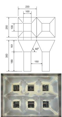
Fig. 3. View of inlet section (Y-chute type)
