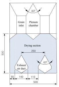
Fig. 2. View of drying section.
