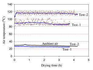
Fig. 6 Average variation of drying air temperature during drying.
