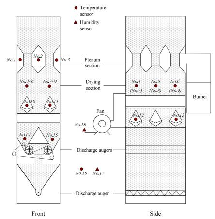
Fig. 5 The positions of temperature and humidity sensors.
