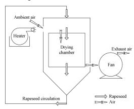
Fig. 1. Block diagram of rapeseed concurrent flow dryer.
