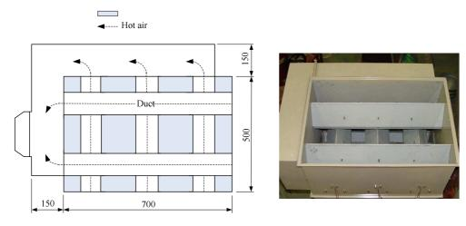
Fig. 4 View of exhaust air ducts.
