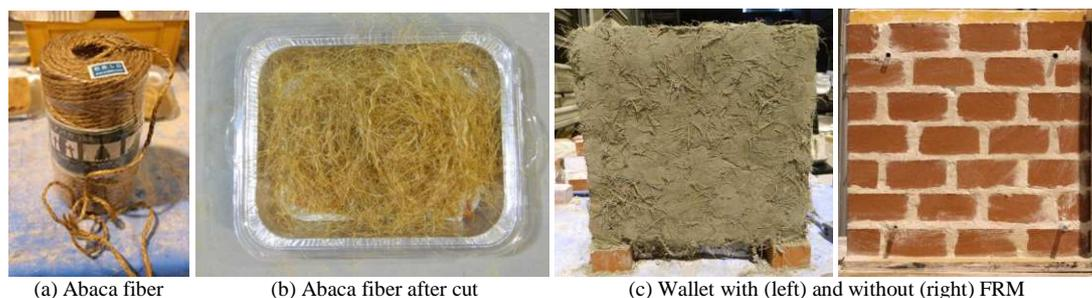
Fig. 1 Photos of specimens (in-plane wallet)
