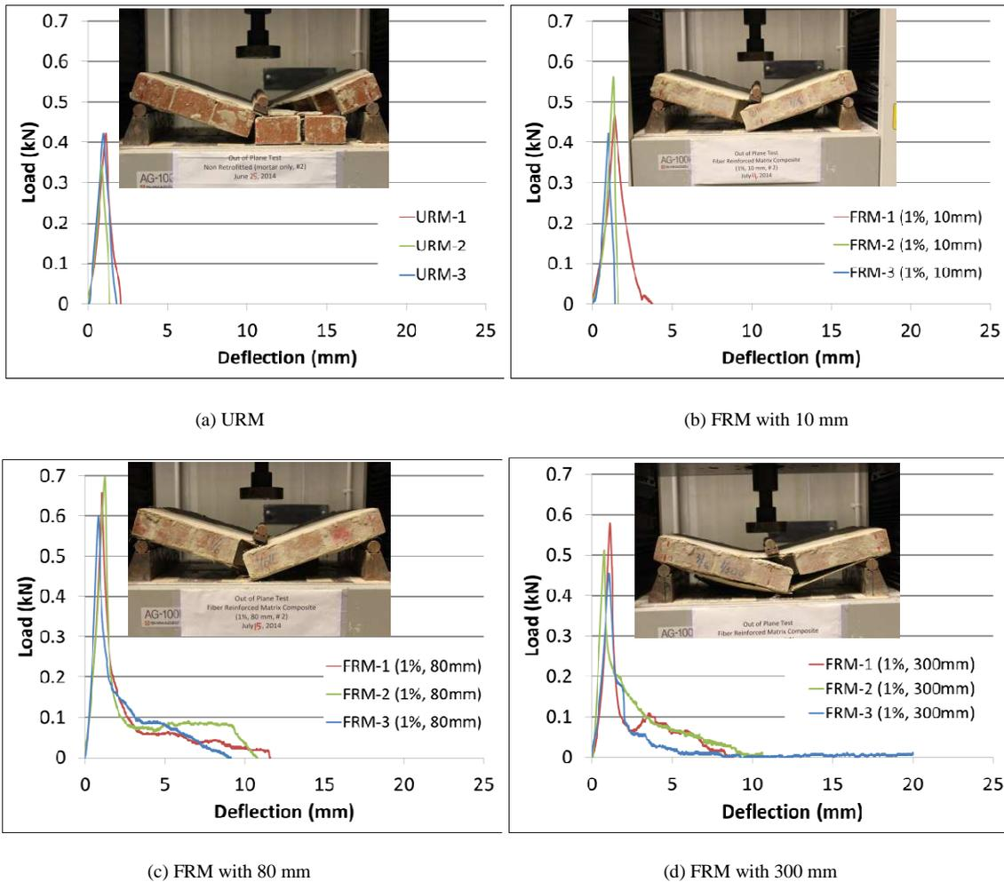
Fig. 6. Load-deformation curves of URM and FRM wallets (out-of-plane test)
