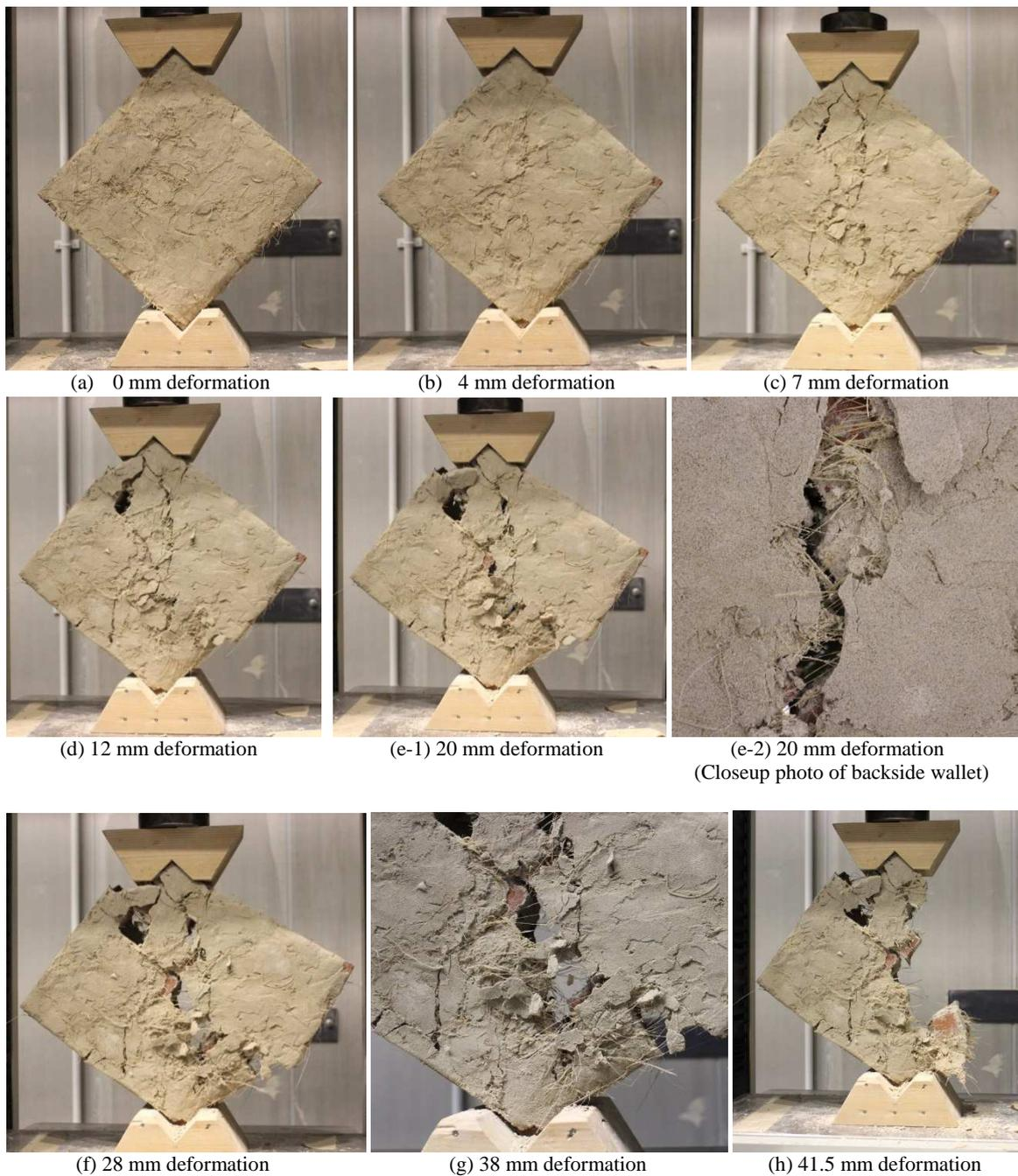
Fig. 7 In-plane testing of FRM wallet with 100 mm fiber length (FRM-1 in Fig. 4 (e)) from (a): the beginning, (b): initial diagonal crack occurred, (c-f): the crack became bigger and other cracks appeared, (d-g): Abaca fiber bridges the crack, and (h): collapsed wallet
