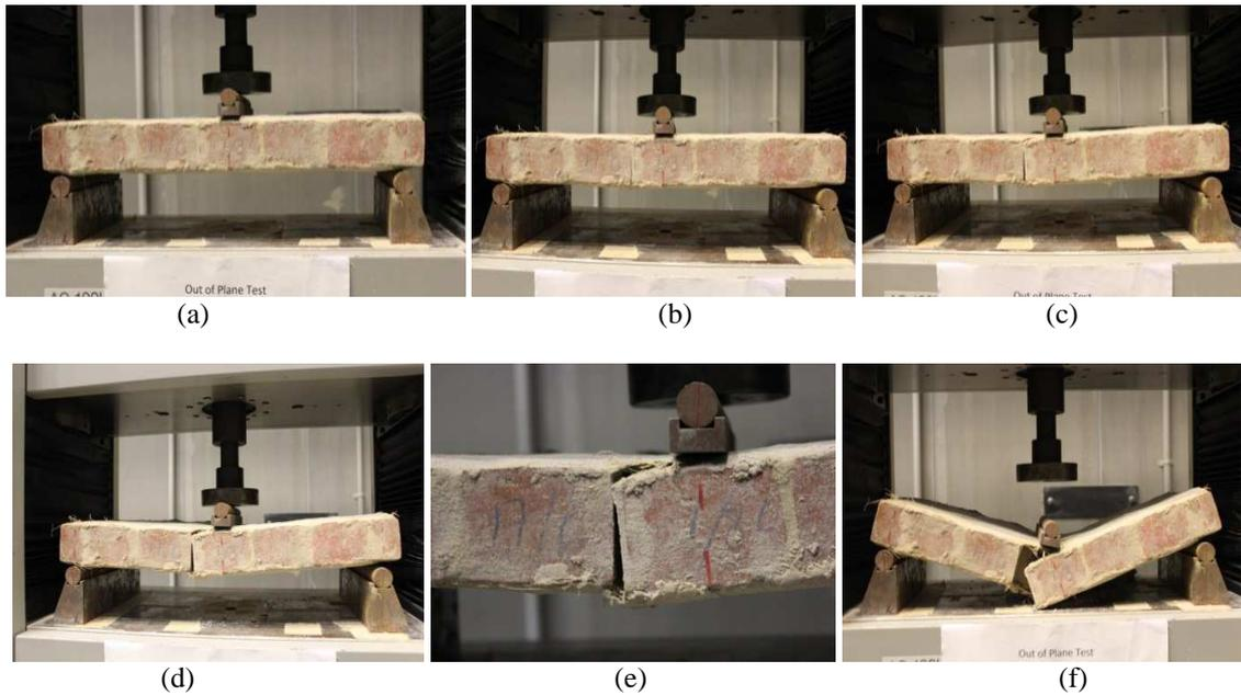
Fig. 8 Out-of-plane test using FRM wallet with Abaca fiber length 80 mm from the beginning (a), initial diagonal crack occurred (b), the crack became bigger (c, d), Abaca fibers bridge the crack (e), collapsed wallet (f)
