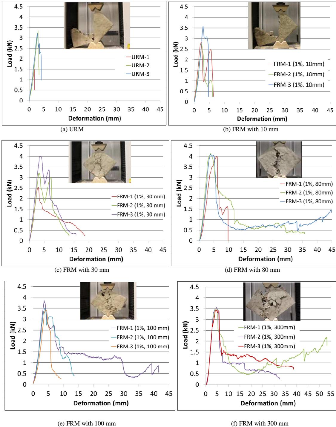
Fig. 5. Load-deformation curves of URM and FRM wallets (in-plane test)
