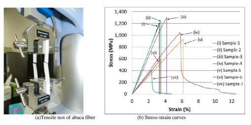
Fig 4. Tensile test of Abaca fiber
