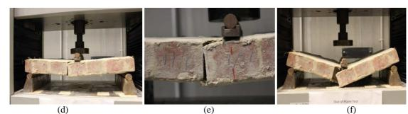
Fig. 8 Out-of-plane test using FRM wallet with Abaca fiber length 80 mm from the beginning (a), initial diagonal crack occurred (b), the crack became bigger (c, d), Abaca fibers bridge the crack (e), collapsed wallet (f)
