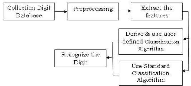
Fig 1: Block diagram proposed handwritten digit recognition system
