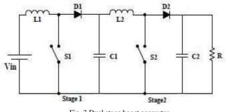
Fig. 3 Dual stage boost converter
