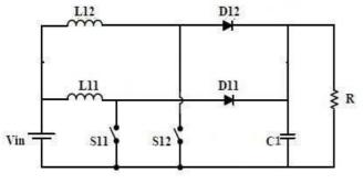
Fig. 1 Dual phase boost converter
