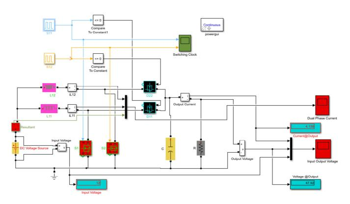
Fig. 7 Simulink Model of Dual Phase Boost Converter
