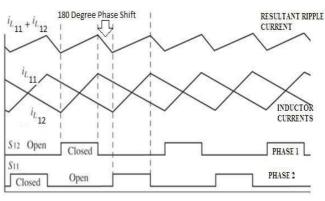
Fig. 2 Dual phase inductor and resultant current
