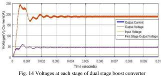
Fig. 14 Voltages at each stage of dual stage boost converter
