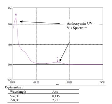
Fig 1. UV-Vis spectra of the sample solution at a wavelength of 540 nm
