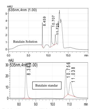
Fig 2. Betalain separation on HPLC chromatogram obtained from a sample solution compared with standard betalain chromatogram  $\,$
