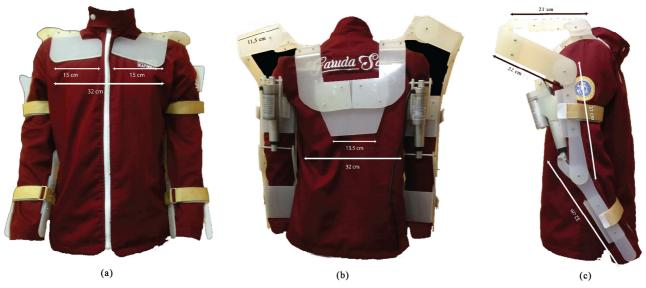
Fig. 1 The Exoskeleton of post-stroke rehabilitation device (a) front (b) back (c) lef/right
