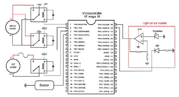
Fig. 5 The layout of the electronic control
