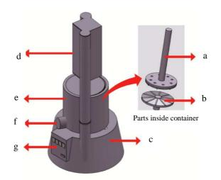
Fig. 2 3D Model of Green Grass Jelly Squeezer. (a) Upper squeezer (b) Bottom squeezer (c) AC motor (d) Servomotor (e) Container (f) Sensor module (g) Power button and speed controller
