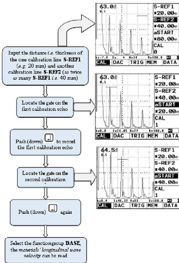
Fig. 2 Simplified M2P procedure on GE USM 35X to obtain materials' longitudinal velocity
