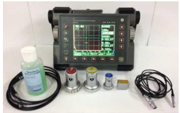
Fig. 1 the Ultrasonic equipment of GE USM35X series [20]
