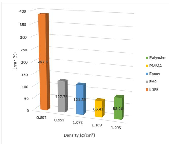
Fig. 4 Results comparison between error and density of polymers at 1 MHz frequency
