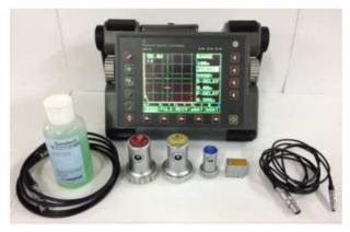
Fig. 1 the Ultrasonic equipment of GE USM35X series [20]
