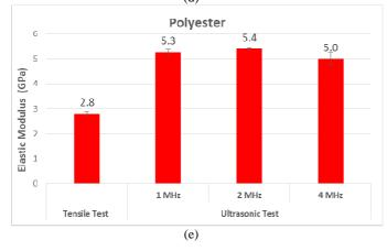
Fig. 3 Comparison between elastic modulus value from tensile test and ultrasonic test; (a) PMMA, (b) PA6, (c) LDPE, (d) Epoxy, (e) Polyester
