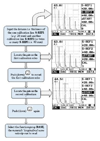
Fig. 2 Simplified M2P procedure on GE USM 35X to obtain materials' longitudinal velocity
