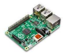
Fig.4 PC board Raspberry Pi3
